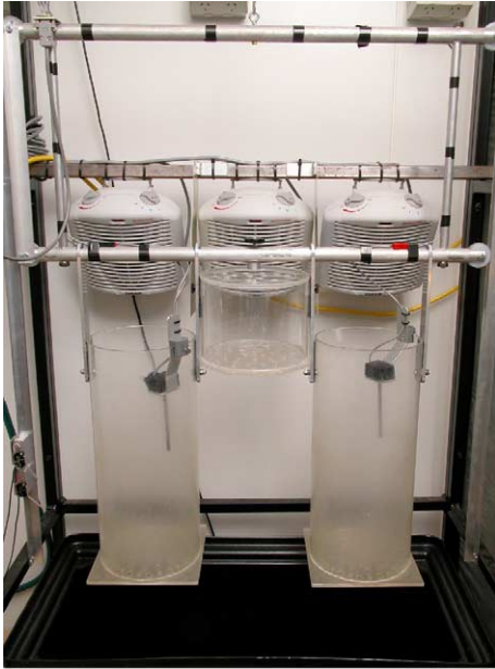
Fig. 1. A picture of the swim stress controllability apparatus. There is an escape rat (left cylinder) that can terminate the forced swim by pressing an omnidirectional lever, a yoked-inescapable stress rat (right cylinder) that has no control over the duration of the forced swim and a confined rat (middle cylinder). The confined rat remains in the apparatus for the same period of time as the 2 swim stressed rats, is exposed to the same handling and movement, but is not exposed to the water. A fourth rat remains in the vivarium (home cage) during the stress session.
